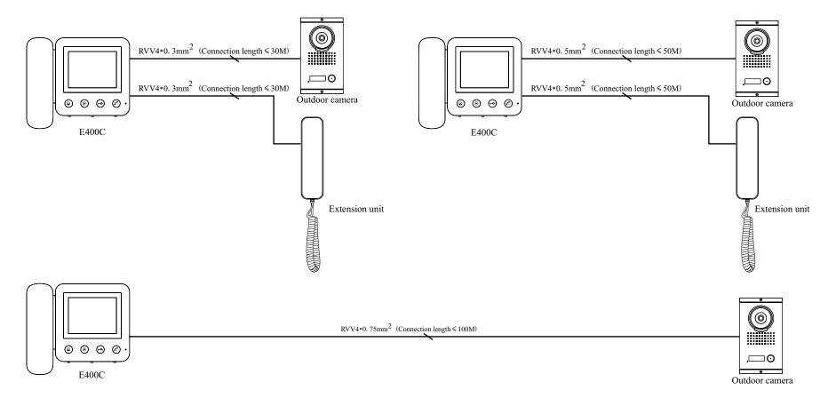
The wire's specific resistance should be ≤0.06 ohm/m.
