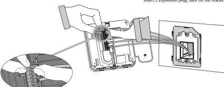
3. Connect the wire to each connection terminal, then check if the wire is fixed enough. (see the wiring sequence on the picture)
