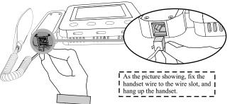
5.Insert the handset wire to the wire slot.(attention: model E706 pass this step.)
